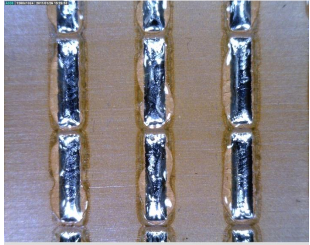
Figure 3b. Wetting pattern for testing for Sn992
