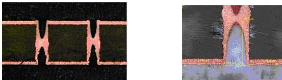
Fig 7: 400 µm thick core with 100 µm TH plated within 15 min. Right detail showing 9 µm plated Cu on the surface while > 50 µm Cu plated in the middle of the via
