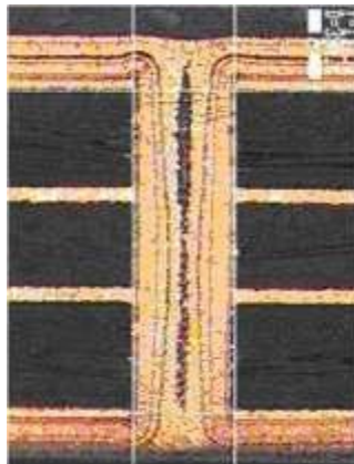
Fig. 2: Conformal Cu growth to a complete fill may end up in producing a long ribbon like void
