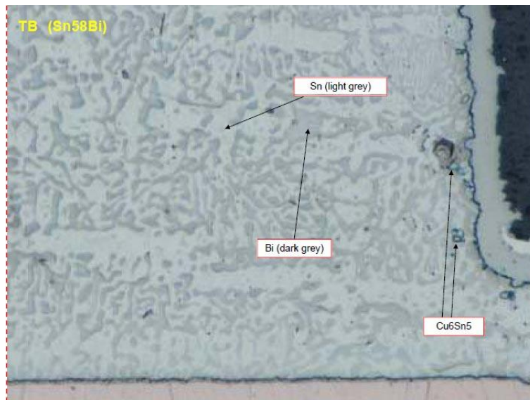
Figure 27: Sn58Bi soldered 3216 [1206] chip component cross-section.
