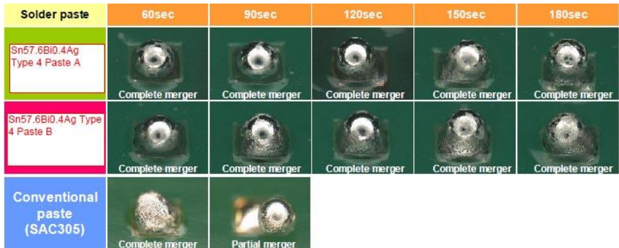
Figure 17: SnBi0.4Ag Type 4 paste A versus SnBi0.4Ag Type 4 paste B versus Sn3Ag0.5Cu paste C head-in-pillow testing.
