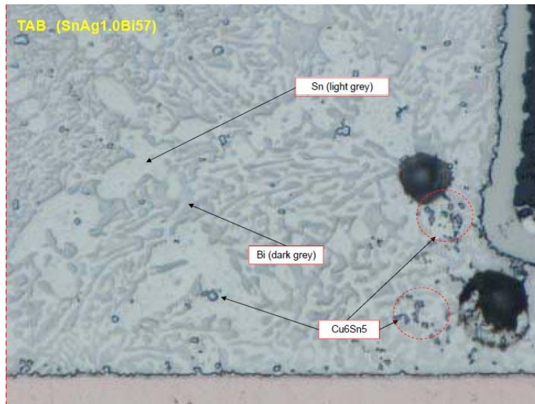
Figure 29: Sn57Bi1Ag soldered 3216[1206] chip component cross-section.
