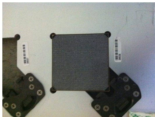
Figure 5 – Close up view of Fixture for automated 3D X-Ray inspection
