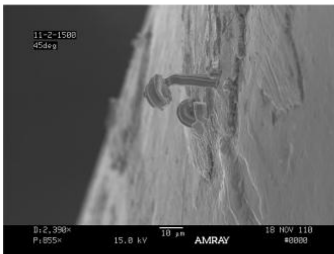
Figure 14: Typical Tin Whisker Observation (Test Specimen #11) during 1500 Hour Inspection Interval
