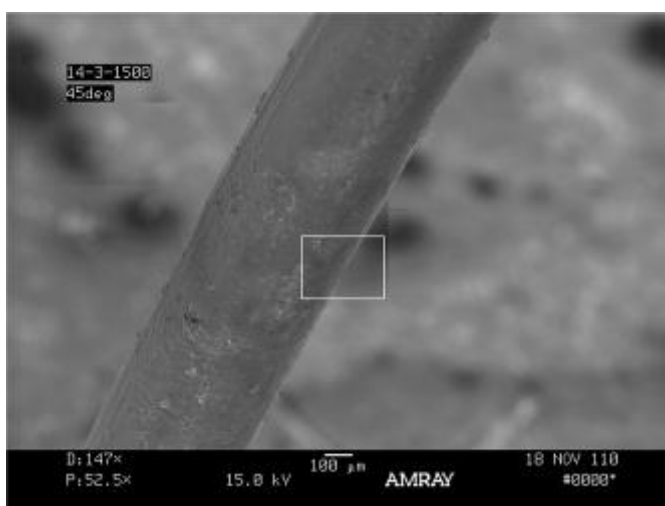
Figure 16: Typical Tin Whisker Observation (Test Specimen #14) during 1500 Hour Inspection Interval
