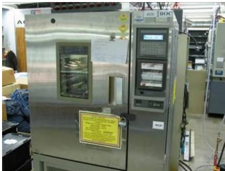
Figure 2 Conditioning Chambers: High Temperature/Humidity
