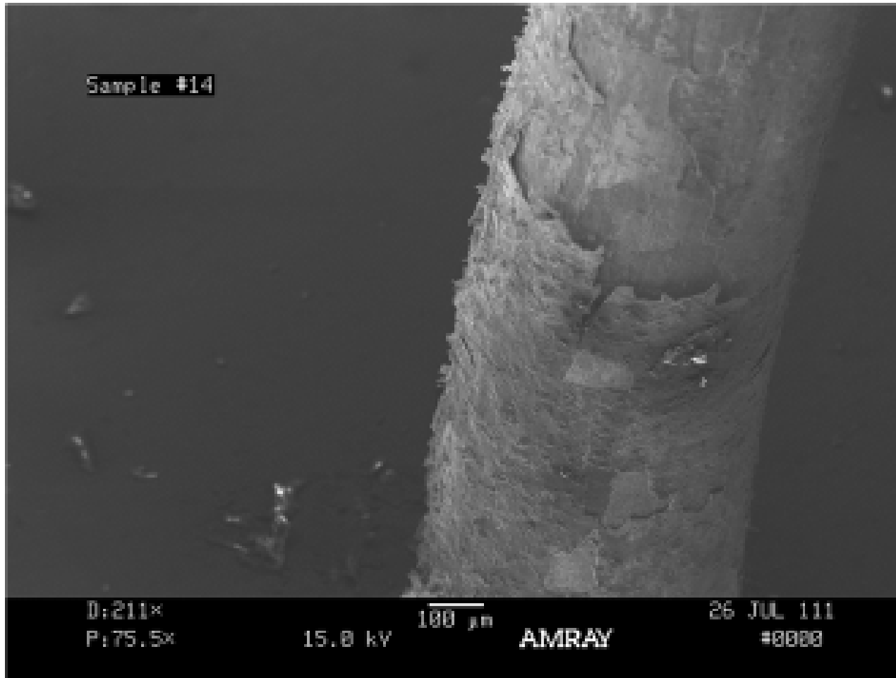
Degradation of plating on specimen 14
