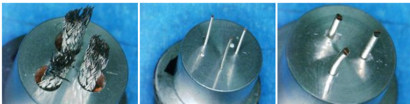
Figure 1: Examples of Test Specimens in Aluminum Specimen Holders Ready for Inspection
