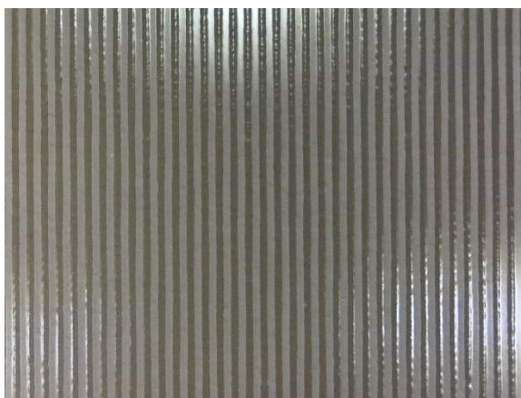
Figure 22 - Microscope photo of 0.004" printed silver lines with 0.006" gap in-between
