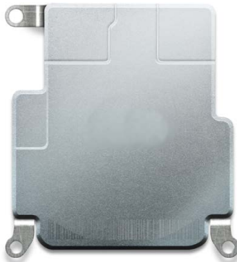
Figure 1 – Example SiP Unit with Sputter Coating and Integrated EMI Shielding Structures
