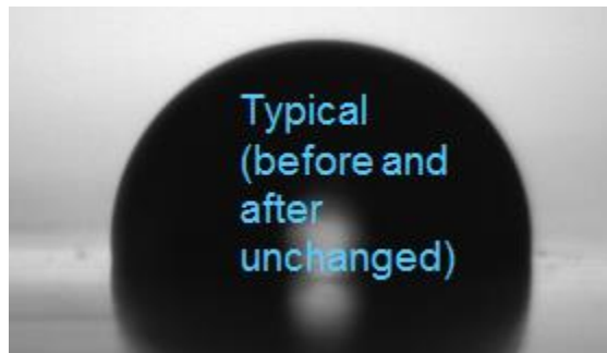
Figure 4 – Representative Photograph of a Water Droplet on a treated PCB surface.
