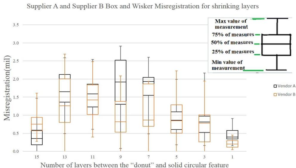
**Figure 5** A box and whisker plot showing calculated misregistration between supplier A and supplier B for shrinking layers.
