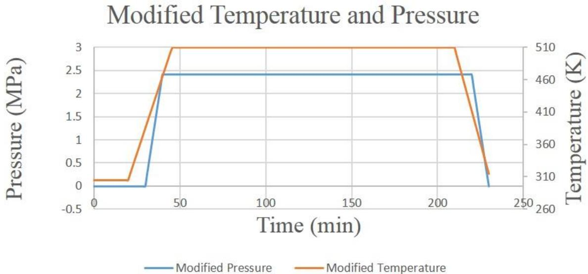
**Figure 14 A modified lamination profile.**
