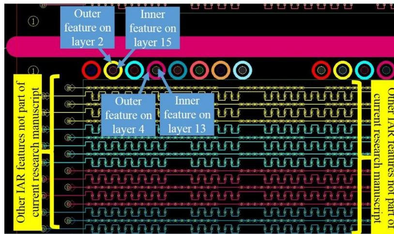
**Figure 3** A screen snapshot of the design file used in test board fabrication. The snapshot shows the location and shape of the test features discussed in this research manuscript.
