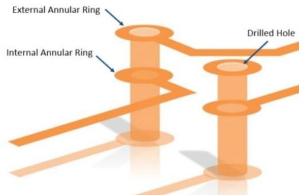
**Figure 2** Schematic illustration of a printed circuit board showing internal annular rings[13].
