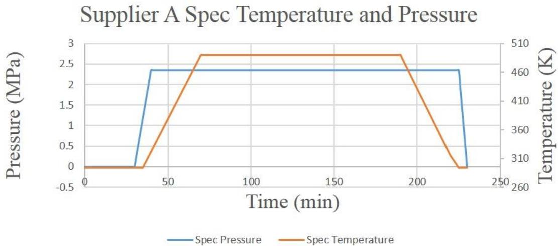
**Figure 11 Lamination profile proposed by manufacturer of material A.**
