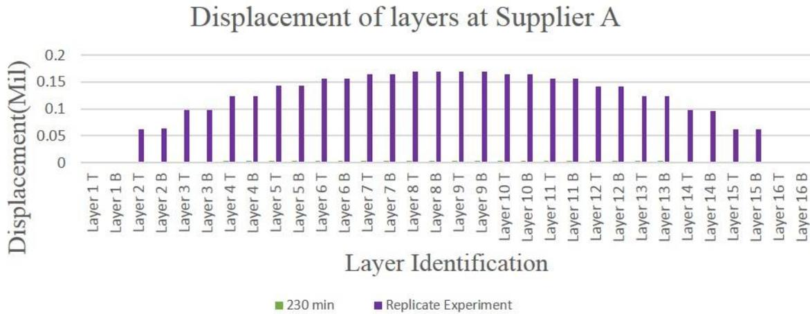
**Figure 15** Displacements observed after modifying the simulated lamination profiles used in the FEA model.
