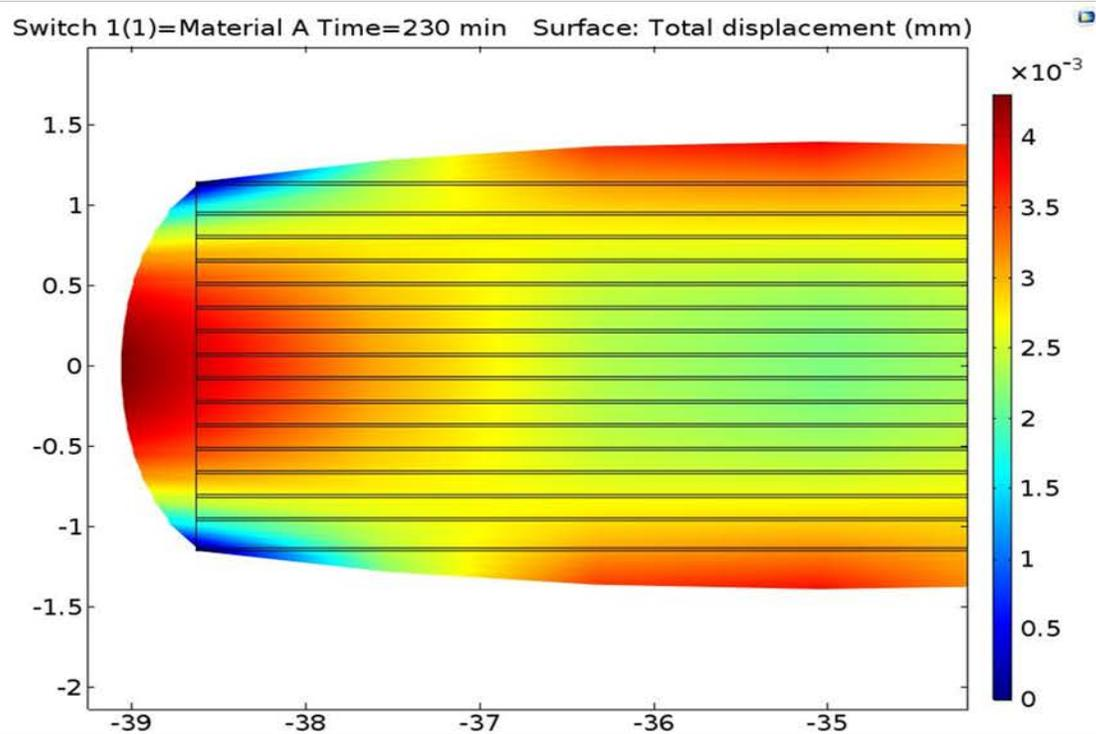
*FEA model output showing calculated displacements.*
