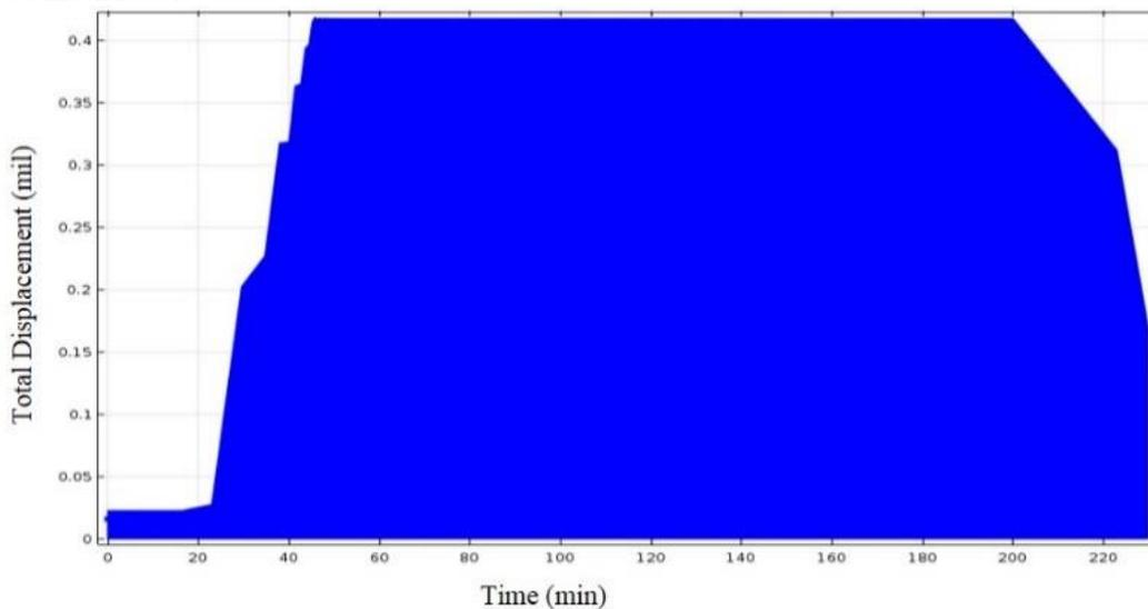
**Figure 16** Displacements within the PCB layer, observed after the inputs into the FEA model were adjusted.
