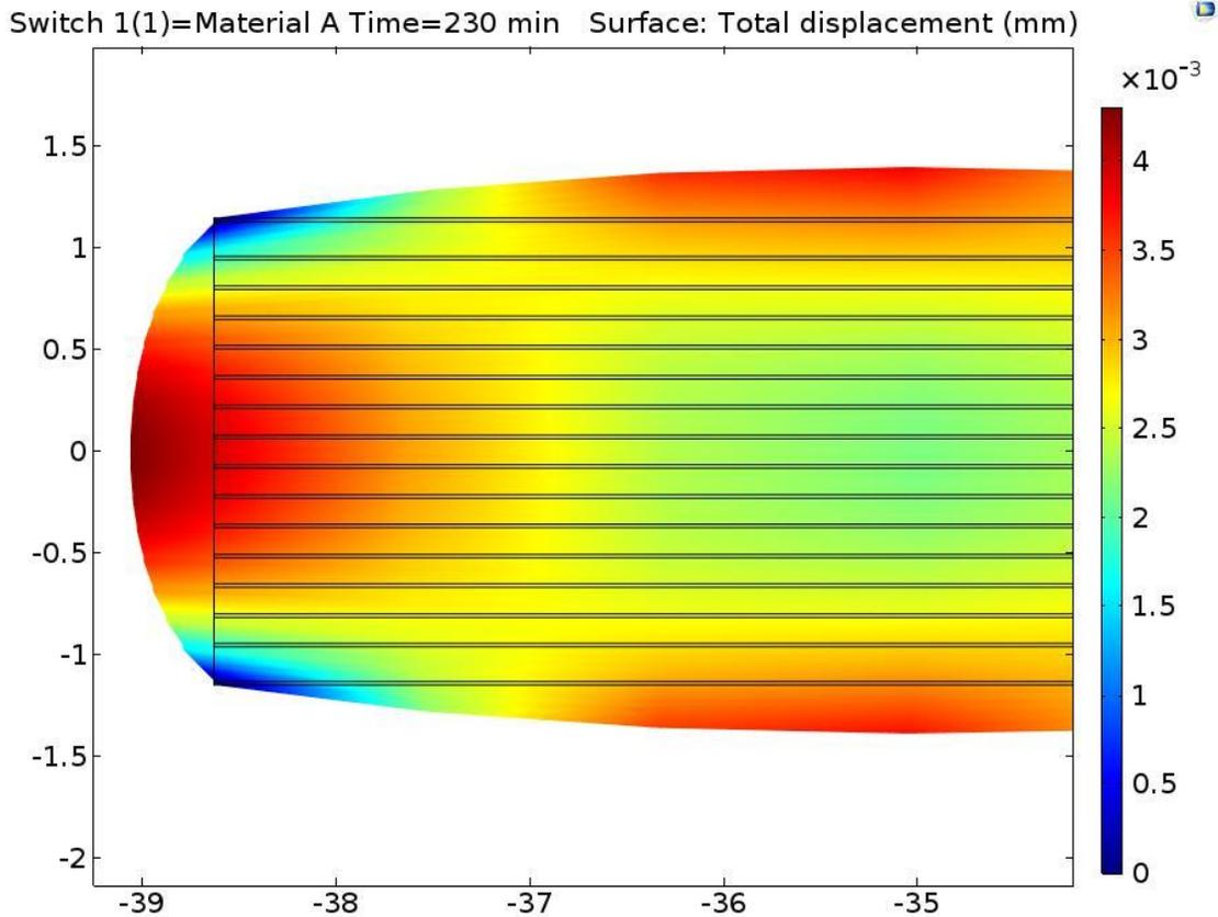
Figure 9 FEA model output showing calculated displacements.
