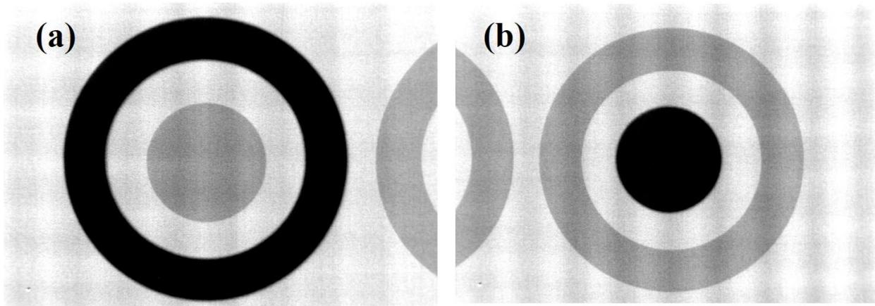
**Figure 4** Sample x-ray radiographs obtained on the test boards. Similar radiographs were observed at each test pattern location on each of the forty test boards. Radiograph (a) shows a donut pattern that was designed on layer 2 and an inner solid pattern on layer 15. Radiograph (b) shows a similar pattern where the outer donut is designed on layer 15 and the inner solid pattern is designed on layer 2.
