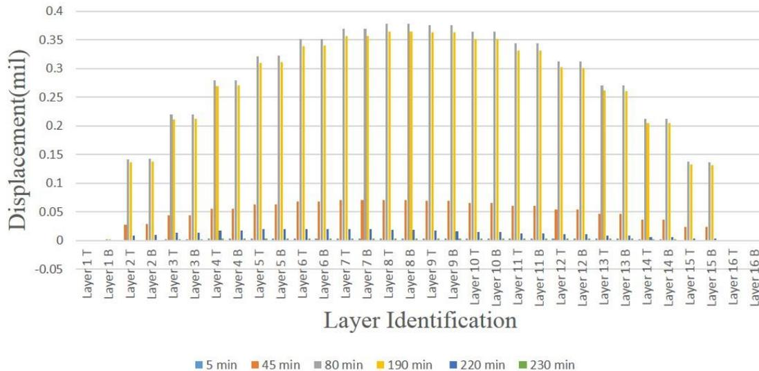
**Figure 12** Displacements obtained from the FEA model after inputting the lamination profile suggested by the laminate supplier for material A.
