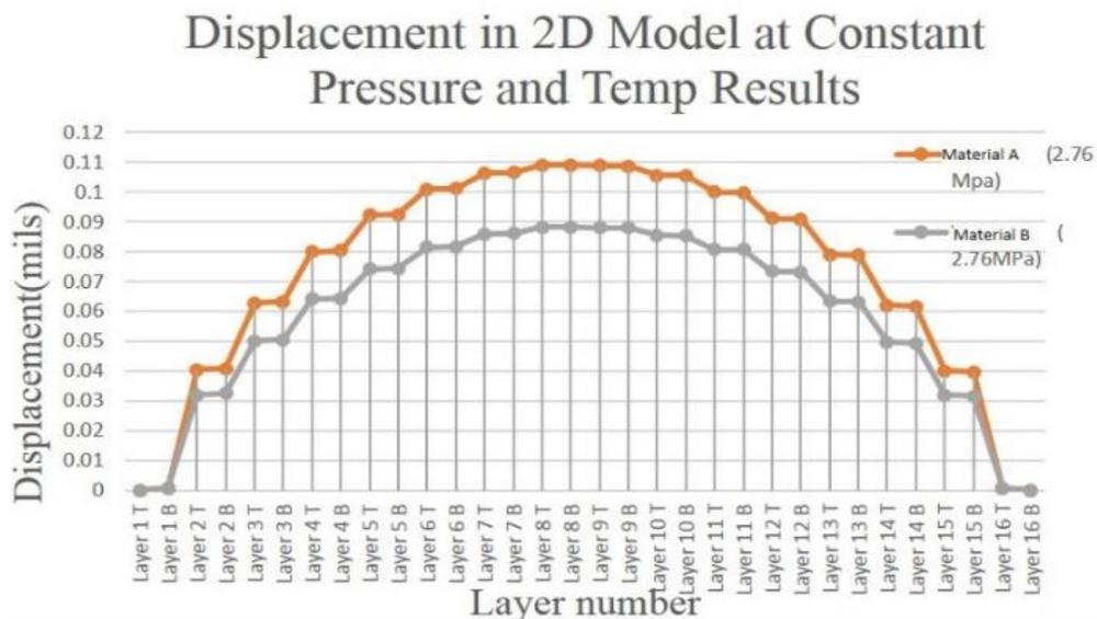
Figure 10 Displacement in 2D at constant pressure and temperature.
