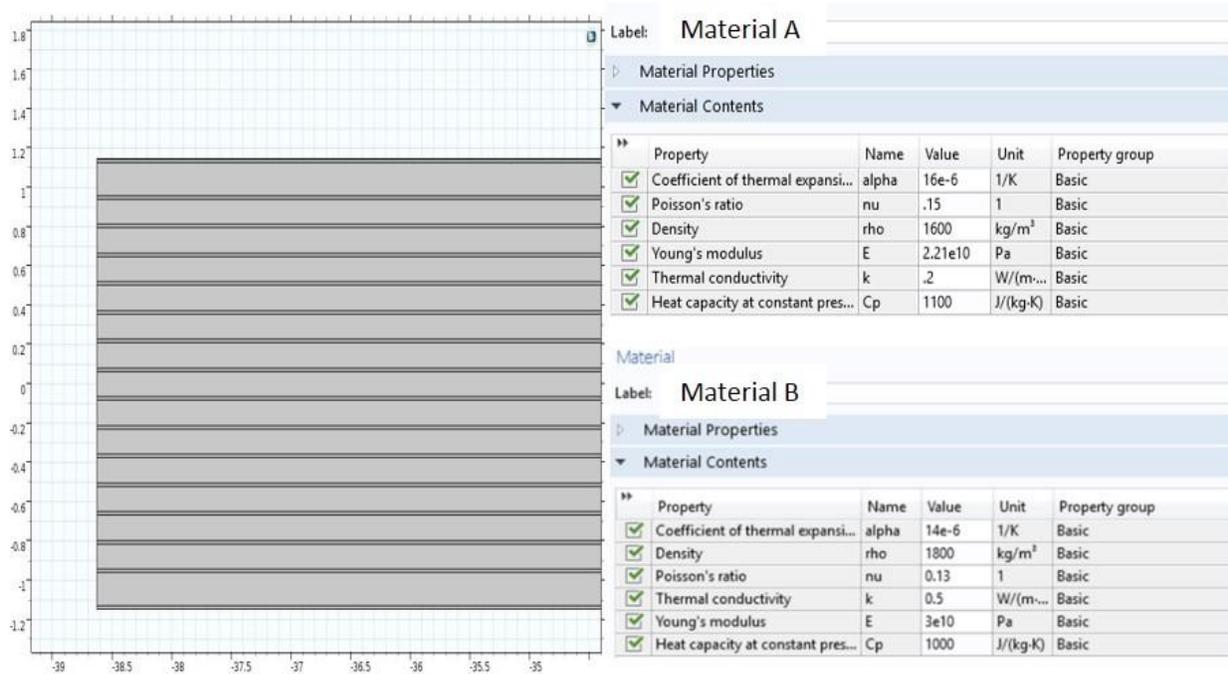
**Figure 8 Geometry of the test sample and model input parameters.**
