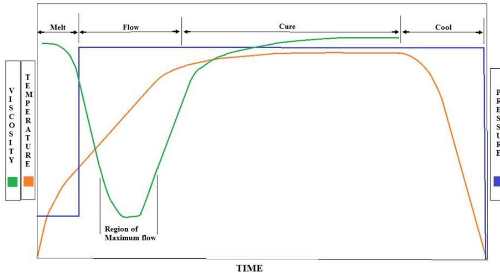
**Figure 1** Overview of the time, temperature and pressure relationship used during the printed circuit board lamination process.
