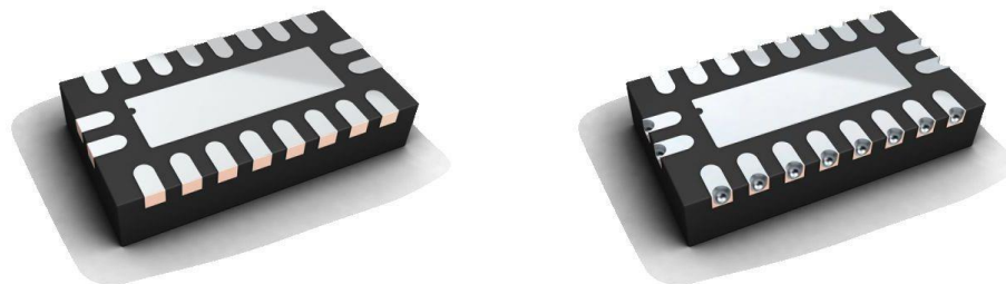
Figure 23: Example of multi I/O DFN/QFN package with dimples to achieve wettable flanks
