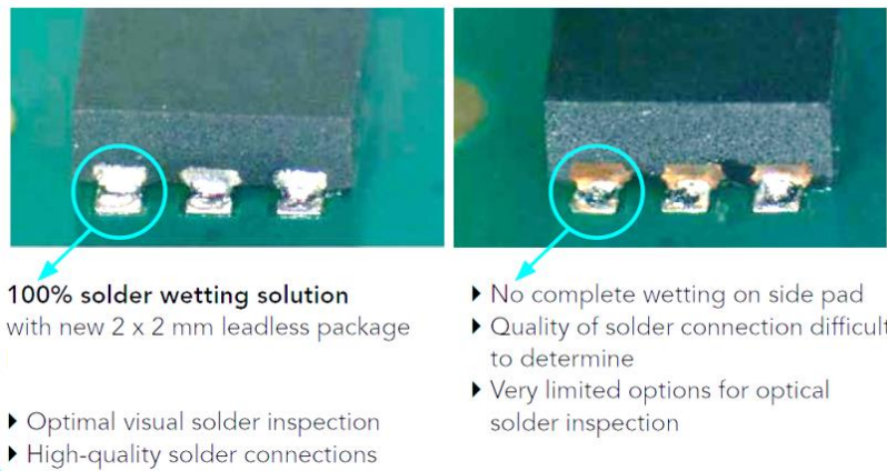
Figure 12: Example DFN2020-6 comparison of SWF versus bare Cu side flanks after soldering
