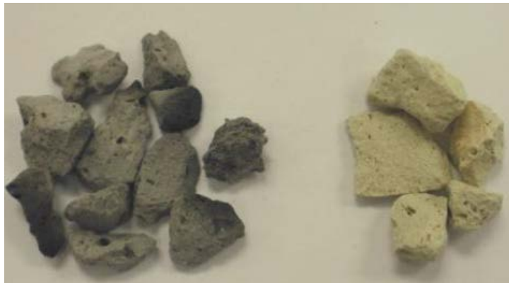
Granulate after and before pyrolysis at 500 °C
