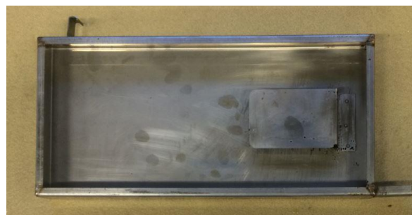
Figure 5: Condensation of ROL0 flux after the catalyst (2 kg)
