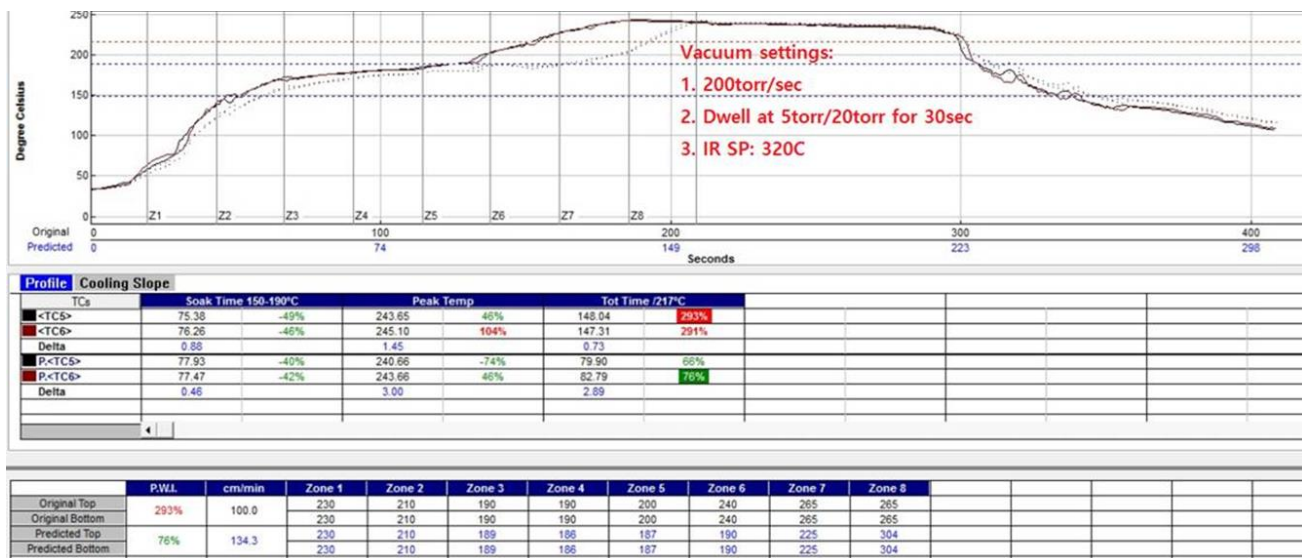
Figure 8- Reflow Profile 1; 30 seconds dwell in vacuum
