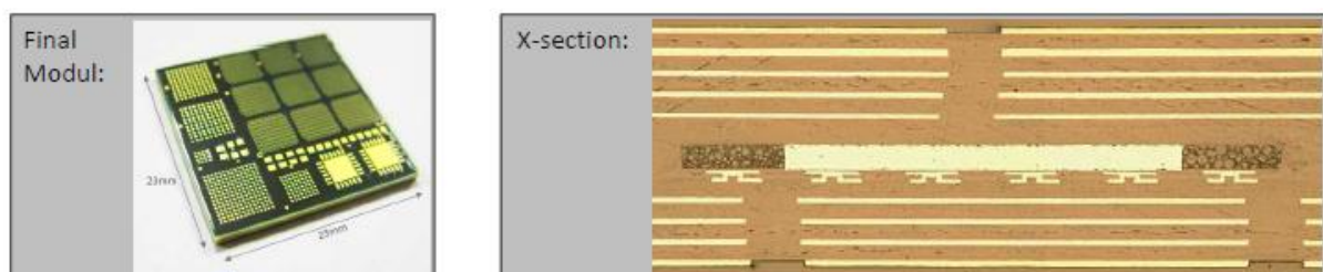
Figure 5 : Realized SoM (System on Module) module and related PCB stacked layer
