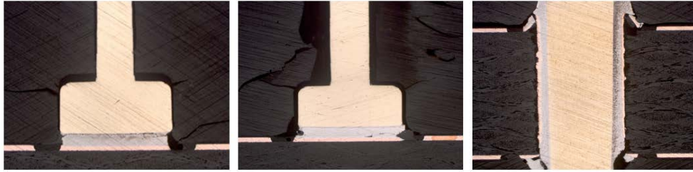
Figure 4 Specimen cycled at 25-125°C thermal cycling showing epoxy separation and cracking around pin flange and ripped copper barrels in through-hole solder joints.
