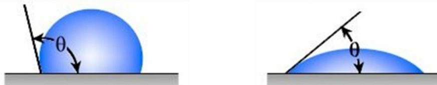
Figure 4: Explanation of Contact Angle and Hydrophobicity
