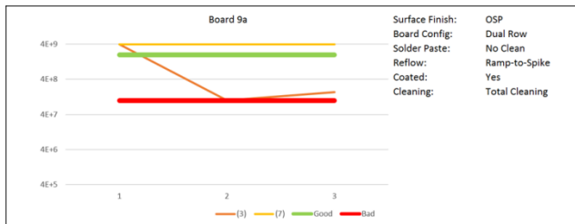
Figure 8: Dual Row Hard Failure at the Unvented Center Lug on Uncleaned, Poly-para-xyleneCoated Board
