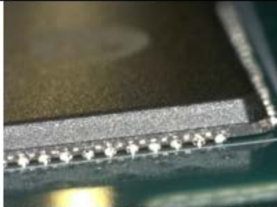
U1: QFN156LD Partially Cleaned
