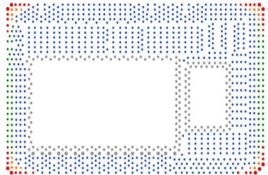
Figure 5 Different colors depict different solder volumes on the same package
