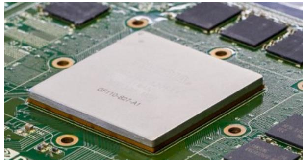
Figure 3 BGA with integral heat sink
