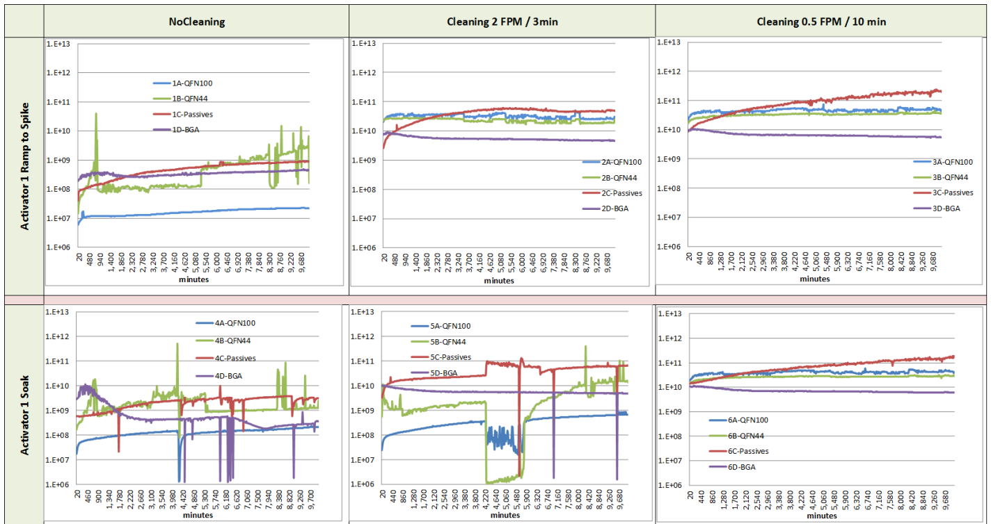
Figure 11: Activator #1 SIR data for Not Cleaned, Partially Cleaned and Totally Clean Test Boards
