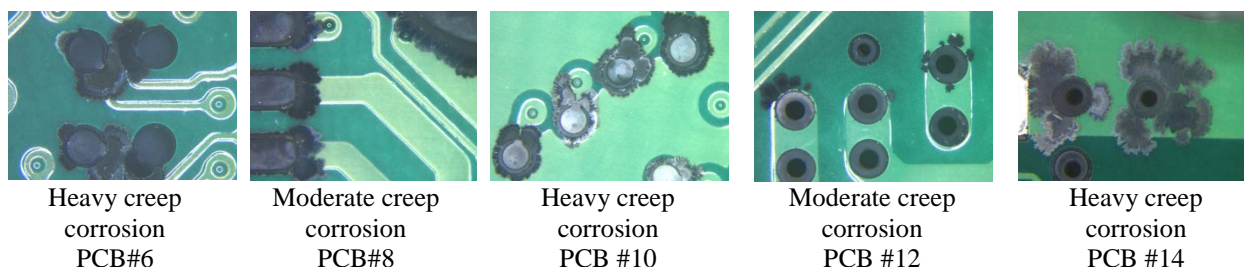
Figure 5: Creep corrosion of five of the seven prebaked PCBs that suffered creep corrosion.
