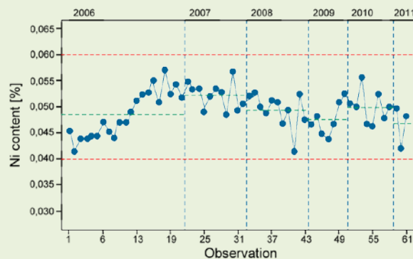
Figure 13 Ni concentration in SN100C alloy used in a wave soldering line producing communication products.
