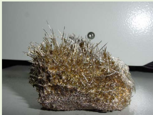
Figure 12. FeSn 2 needles found in a selective solder pot with SAC305 alloy.
