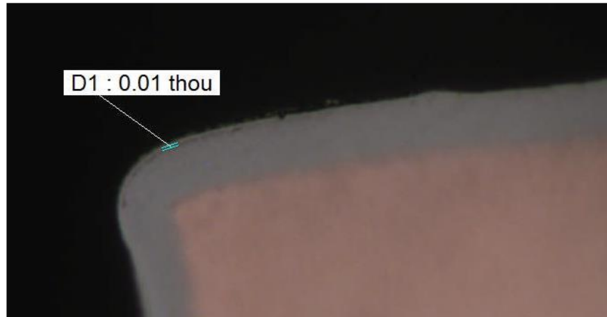
Figure 22 - Edge of the Pad Showing Demarcation Line at 1000x Lens.
