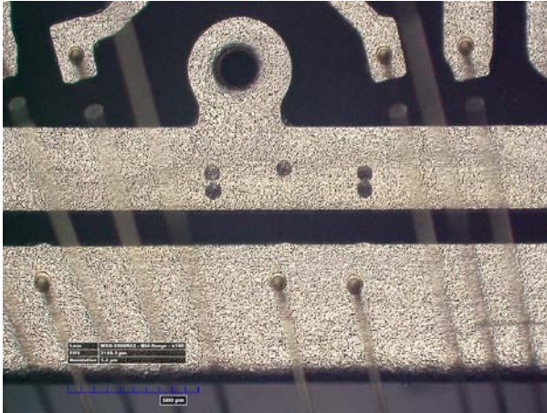
Figure 16 - Five Black Circles Represent PML Including Attempts to Repair
