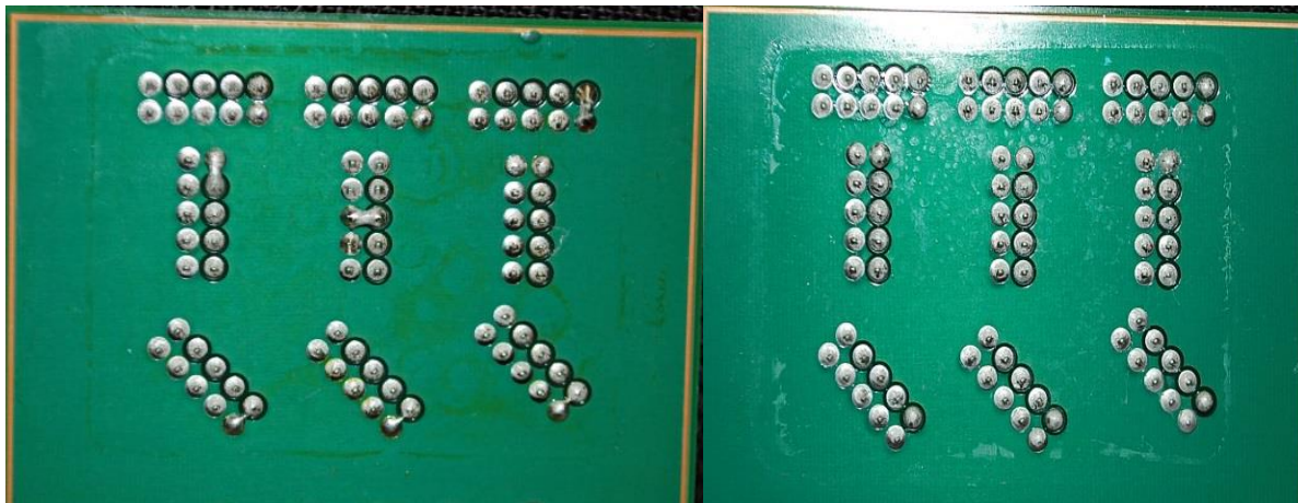
Figure 13. Flux Residue for Flux H and Flux F
