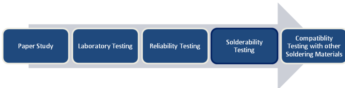
Figure 1. Methodology for Flux Selection
