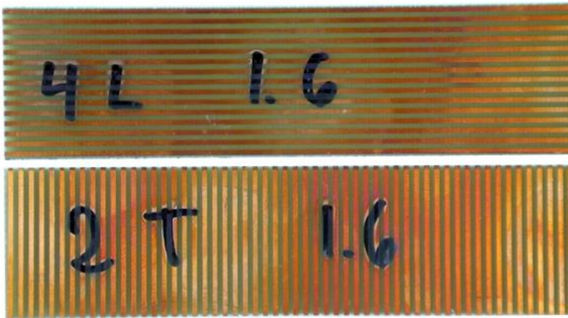
Figure 9–Copper trace direction on test laminates; length direction (top), crosswise direction (bottom) 12 .
