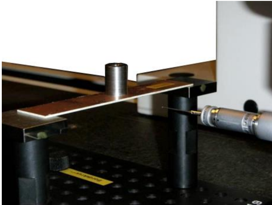
Figure 5 - Measurements of laminate with weight prior to reflow 8
