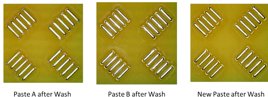
Figure 13 – Flux Residues on Circuit Boards after Washing
