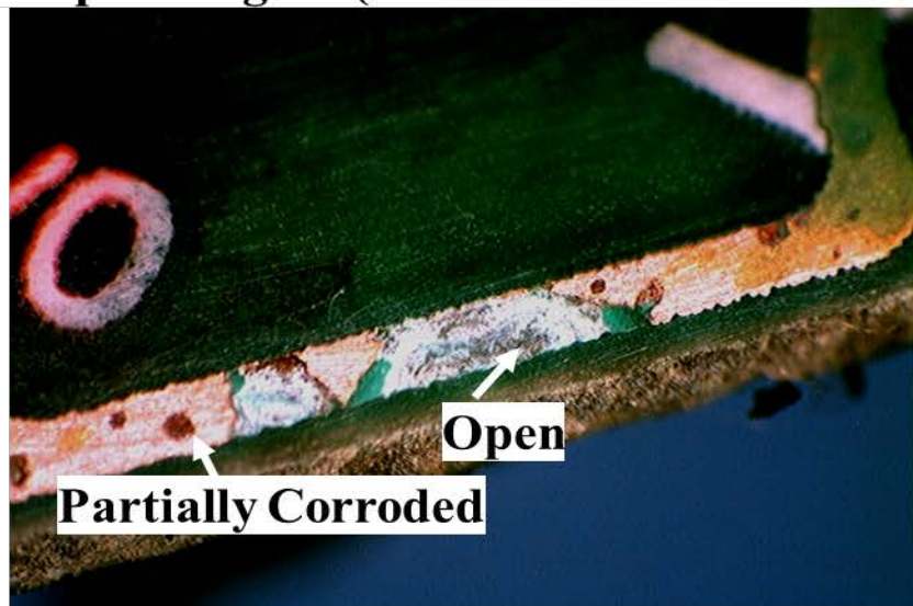
Suspect Region (after soldermask removal)
