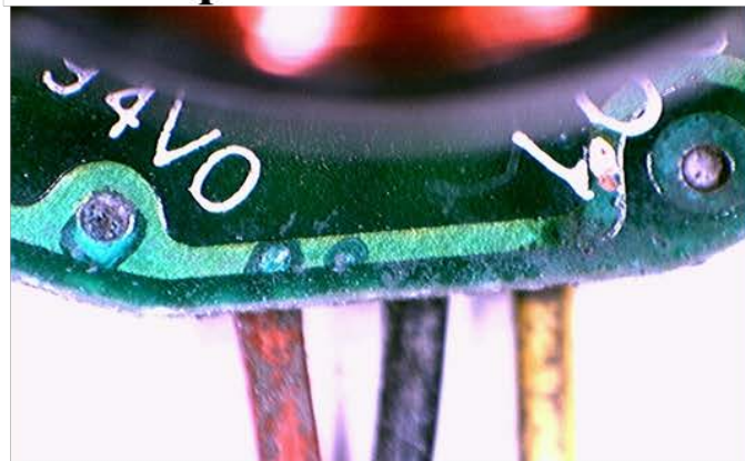
After Tape Lift-off and IPA Clean
