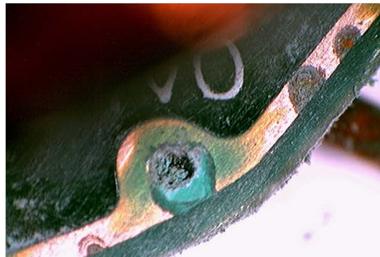
After Cleaning and Sanding with 600 Grit paper
