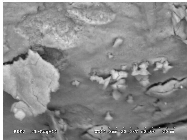
Figure 25: Whiskers at site of oxidation SOT6, contamination condition 1-1
