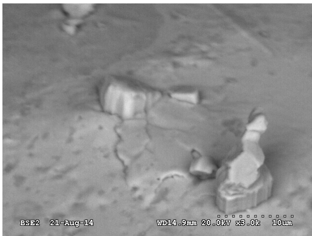
Figure 24: Many short whiskers SOT6, contamination condition 1-1
