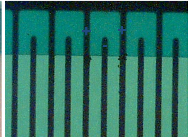
C. QFP80 Comb Possible Dendrites (Backlighting)
