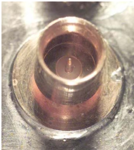
Figure 6. Surface Mount Connector's Center Pin Embrittlement Examination. Connector Top View (Left). 100X Cross-Sectional Views of Failed Pins (Right).
