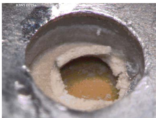
Figure 12. During the Pin Pull Test, the Pin-to-Trace Solder Joint was So Strong that the Trace Pad and the Board Material were Torn Out of the Board.
