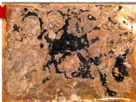
Phase 1 with scrub and acid etch dip
