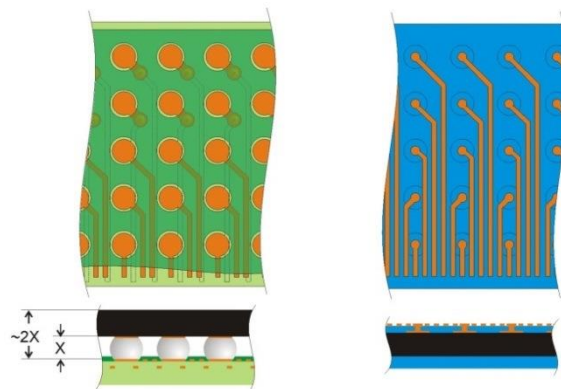
Figure 5 At any given lead pitch, solderless assembly methods can significantly reduce layer count by freeing up routing space as illustrated on the right. The approach provides freedom to use nearly any position within the BGA matrix for routing objects; traces & vias". For example, while via in pad is good. Via wherever (e.g. on pad, off pad, overlapping pad) is even more effective. This added flexibility in routing compliments the trend toward the dominance of ASICs & other System-On-Chip devices. That is it offers more flexibility for more signal pairs, more accordion routes (length matching), shielding, wave guides, etc. Note also that solder balls often makes up half of the overall height of a mounted package, thus a much thinner assembly is possible.
