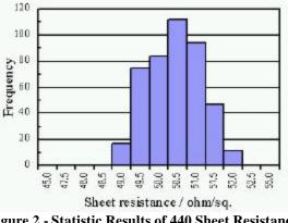
Figure 2 - Statistic Results of 440 Sheet Resistance Measurements on a 500ft Production Roll - NiCr, 500hm/sq. on 1/20z Reverse Treated Foil
