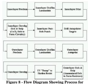
Forming Resistors with TCR Material
