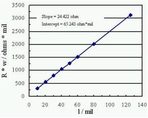
Figure 5 - *Rw* vs. l Plot to Calculate the Total Amount of Resistor Length Compensation - Data are from Table 2, STD Foil - Calculated Total Amount of Resistor Length Compensation is 2.66mil
