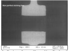
Figure 3 - Resistor Image Shows Non-Perfect Straight Etched Copper and Resistive Edges
