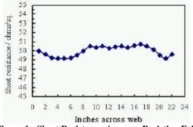
Figure 1 - Sheet Resistance Across a Resistive Foil Web - NiCr, 500hm/sq. on 1/20z Reverse Treated Foil
