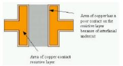
Figure 4 - Illustration of Interfacial Undercut Between Copper and Resistive Layer During Etching
