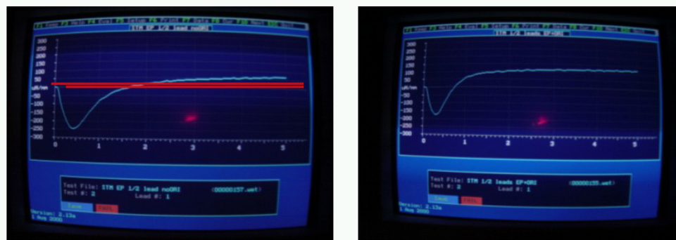
Figure 3 – Wetting Balance Testing: Left – without ORI; Right – with ORI
