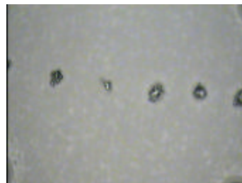
Figure 11 - Solder Paste Deposits after Reflow (Slow Ramp Rate) at 2000ppm
