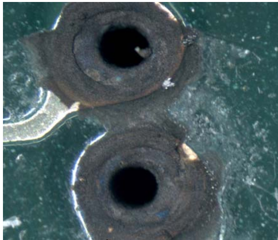
Figure 5 - Test Specimen after 15 Days (>20,000Å) of Class 3 Mixed Flowing Gas under Condensing Humidity (93+/-5% RH) Conditions
