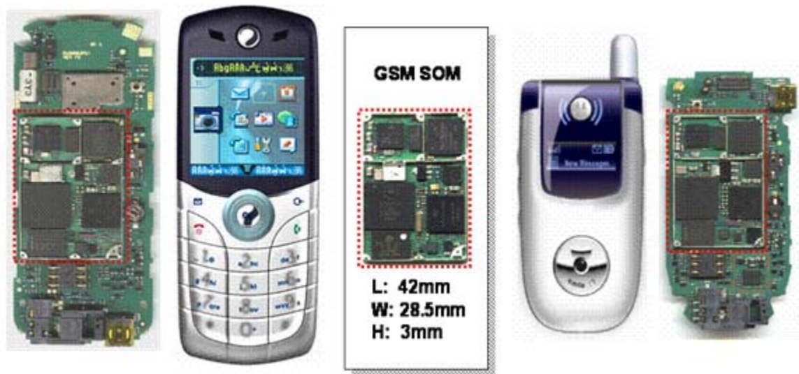
Figure 5 - GSM SOM (center) incorporating the Embedded Mezzanine Capacitor Technology and the C650 (left) and V220 (right) Phones utilizing the GSM SOM
