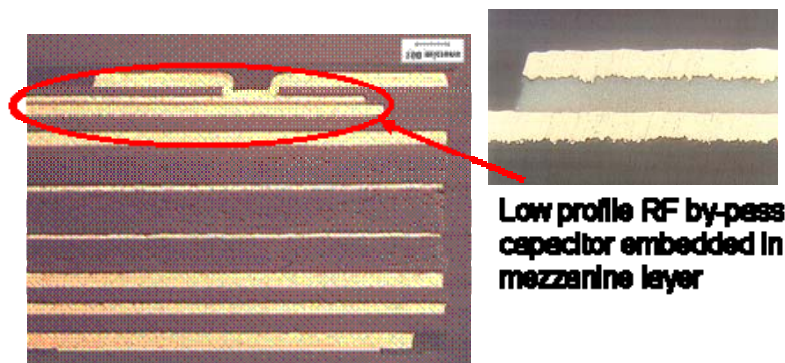
Figure 2 - Mezzanine Capacitor Cross-Section as shown Buried in a Multi-Layer PWB
