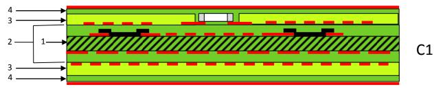
Base-core example with formed passive components in the mounting base and inserted passive components on one side
