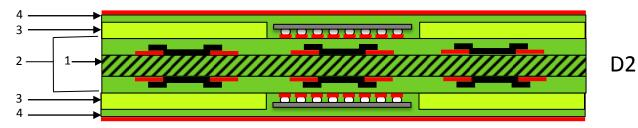
Base-core example with formed passive components in the mounting base and inserted active components on both sides
