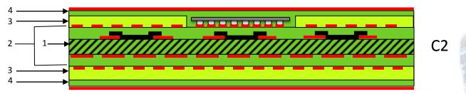
Base-core example with formed passive components in the mounting base and inserted active components on one side
