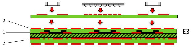
Mounting base example with formed passive components inside the mounting base plus additional layering added to one or both sides to complete the Embedded Component Printed Board ready for component mounting to complete an Embedded Component Board Assembly
