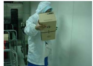
Performed drop test in 10 angles per FSL requirement
