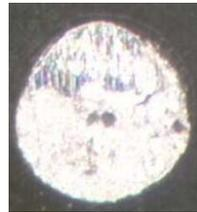
**Figure 6 - Ductile failure mode was observed after ball shear test in all the test conditions.**
