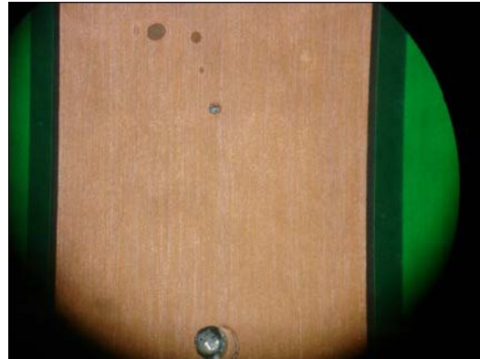
Figure 5 - Inspection point 2 : Left - Reasonable melting of solder dot (n=3); Right - Non-melted solder dot (n=1)
