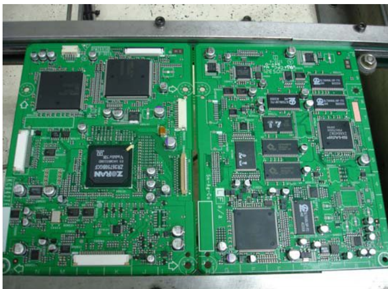
Figure 2 - Test board - 1 st side, immediately before reflow
