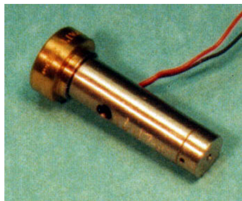
Figure 5 - Single-Jet, High-Temp Printhead (6-mm Diameter)
