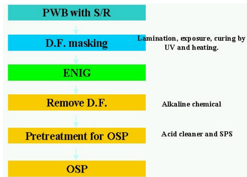
Figure 19 – Process of Selective ENIG for Mobile Phone PWB
