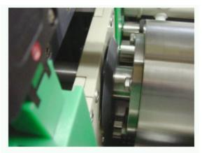
Figure 33 - Brush, Deburr, Nodule Removal
