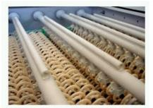
**Figure 7 - Cascading Rinse with Spray Bars** Example: Micro etch developing stripping
