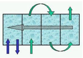
Figure 5 - Separated DI- Water Rinse Last (Final) Rinse
