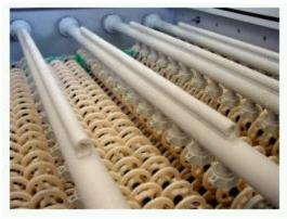
Figure 15 - Rollers staggered
