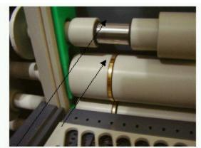
Figure 40 - Insoluble Anodes with Fluid Guide Elements
