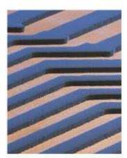
Figure 28 - SEM Lines 40 µm - Very Straight Sidewalls
