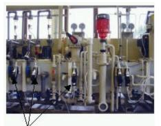
Figure 18 – Pumps Which Can Be Plugged for Quick and Easy Replacement
