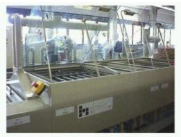
Figure 22 - Double Glass Lids are Used for Security and Cleanness
