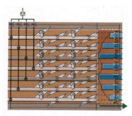
Figure 29 - Flow Control and Adjustment of Individual Spray Bars in Working Direction
