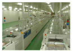
Figure 38 - 2 Fully Integrated Lines: Deburr / Desmear / Electroless
