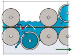
Figure 7 - Rollers Build a Trap and Make the Fluid Go Up and Down (Push – Pull) Through the Holes
