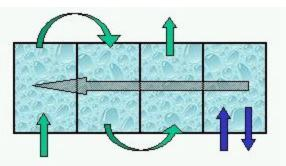
Figure 6 - Separated Concentrate rinse - First Rinse after Chemical Process for Extra Waste Treatment
