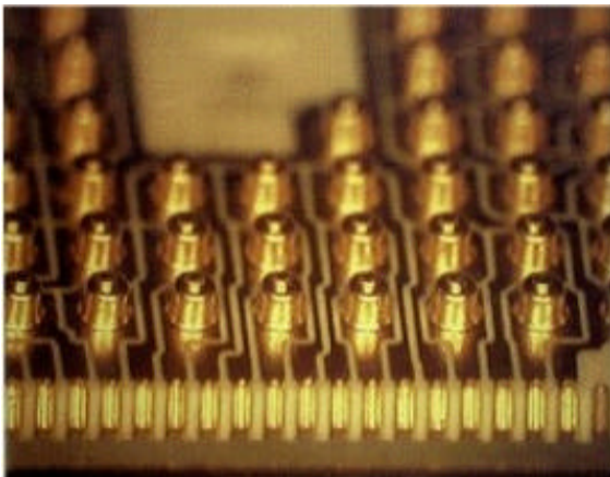
Figure 24 - Example of 3D Laser Structuring on a PSGA –The Laser Tracks are Going Over the Edge
