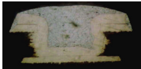
Figure 9 - Electroplated Solder Filled Blind Microvia in Non-Woven Aramid
