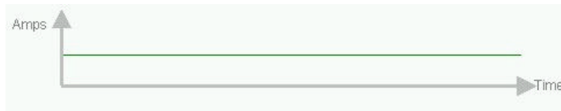
Figure 1– Direct Current Waveform (DC)
