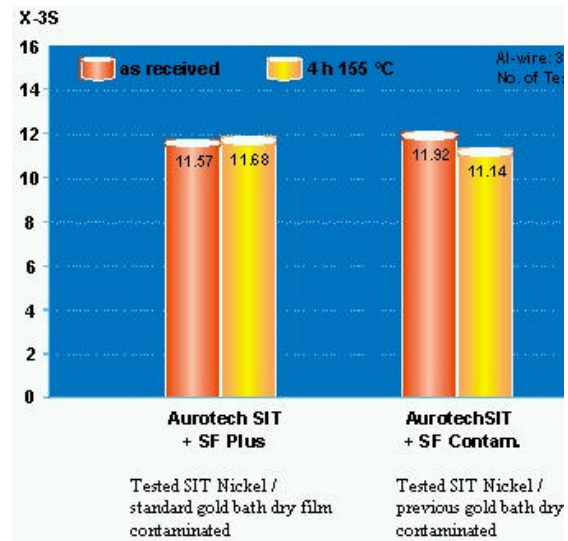
Figure 19 - Al-wire Bonding Pull Forces, for Tested SIT Comparing two Different Gold Baths – Dry Film Contaminated
