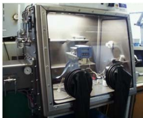
Figure 1 - Glove Box with Solderability Tester
