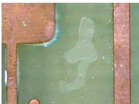
Figure 8 - Blister Spot at the Substrate/Coating Interface of an Acrylic Coated PG7-6 Coupon
