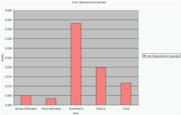
Figure 6 - Actual Cost Per Part Placed is an Extreme Unit Cost Expense when Considered Against Automated Alternatives.
