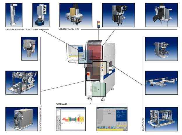
Figure 1 - High Levels of Configureability and Reconfigureability Exist with Today's Automation Systems. This is Facilitated by a Move Away From Robotics Style Controllers and Toward Standard Operating systems and hardware
