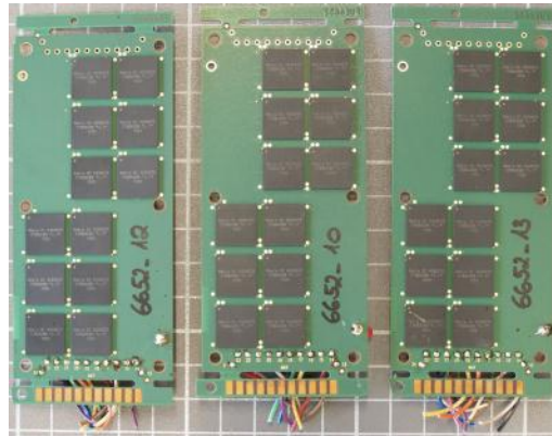
Figure 10: Assembled coupons (TV1) for thermo cycle testing
