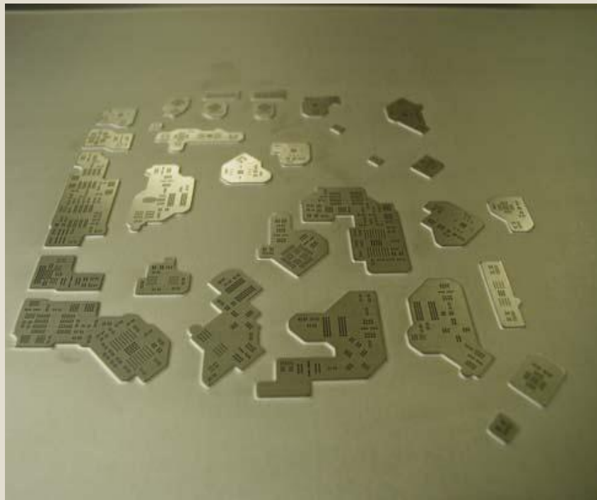
Contact Side view of Paste Reservoir Stencil
